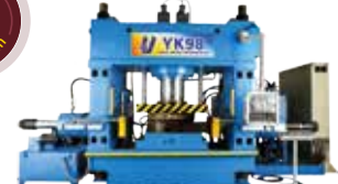
PIPE FITTINGS HYDROFORMING MACHINE
